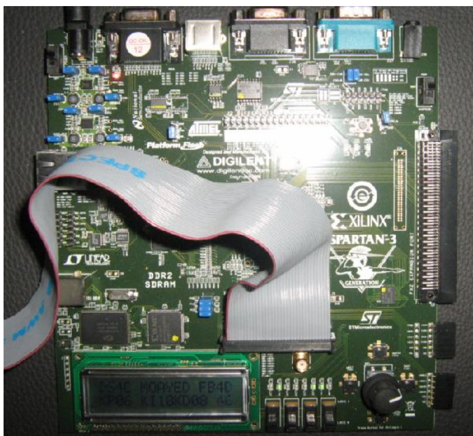
Figure 5.34: PID parameters on FPGA card.
