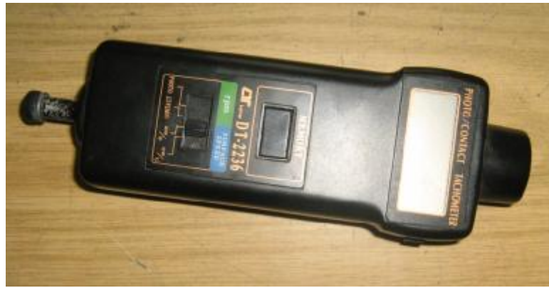
Figure 5.53: Tachometer for speed scaling.
